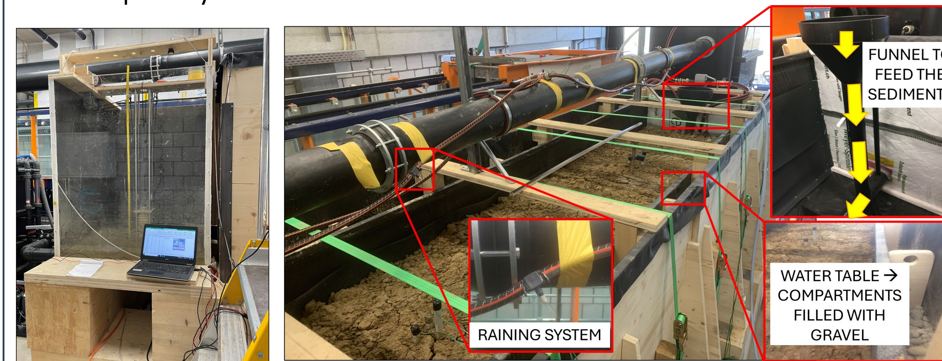
Figure 4: On the left the manhole and on the right the model in the FHNW laboratory
