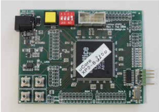
Figure 4: The MicroCore development board. The large chip is the Lattice LFXP2-17E-5Q208C FPGA into which we implemented the different versions of MicroCore. Size: 94 x 70 mm.
