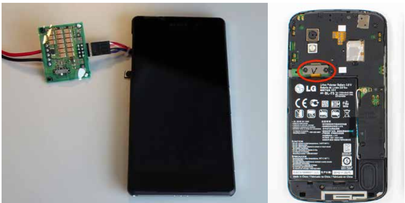
Figure 1: left) Electronic interface to read out power consumption of a smartphone. right) Nexus 4 with an open back cover for connecting measurement equipment.
