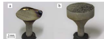
Fig. 3: a) Standard laser parameter: Overheated, incomplete part, b) optimized laser parameter: complete part.
