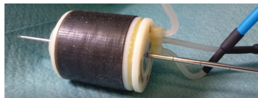
Fig. 2: 3D printed multimaterial pneumatic medical biopsy actuator after gamma irradiation.
