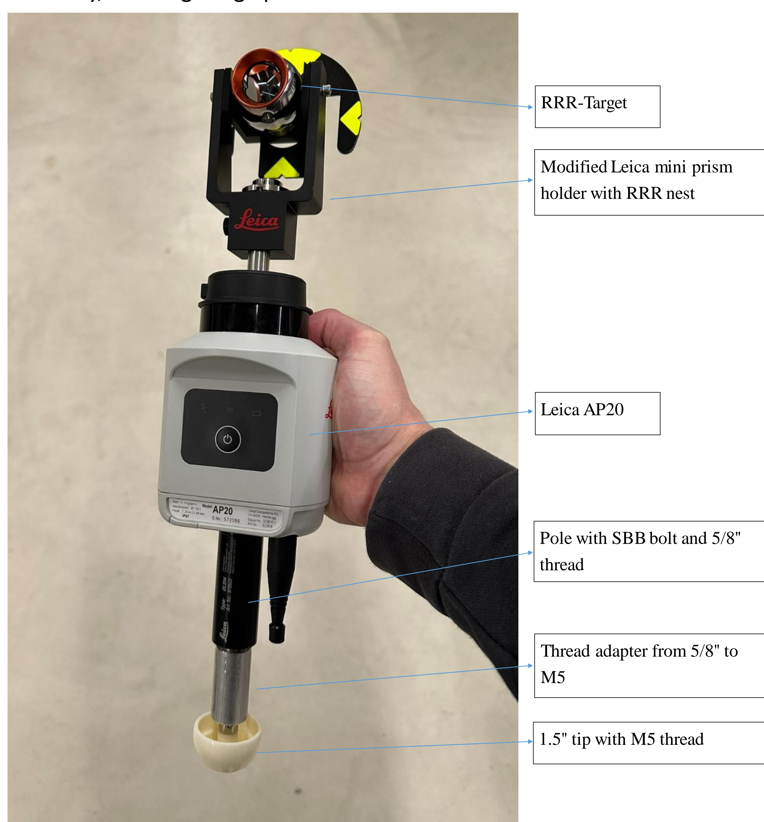
Fig. 1: First prototype of a long-range probe with integrated IMU of the AP20 (short pole)
