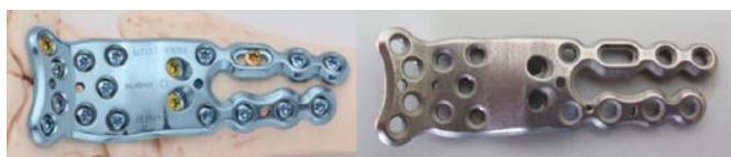
Fig. 1: Left: Medartis wrist fusion plate spanning the radio-carpal and mid-carpal joint. Right: SLM replica.
