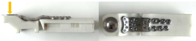
Fig. 2: Wrist fusion plate mounted on the simplified wrist model for dynamic load (arrow) testing.
